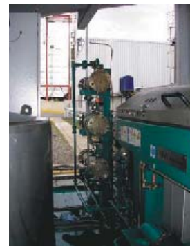
ESSORP -Ultrasonic-Technology with downstream 3-Phase-Decanter for separation of oil, water & solids
