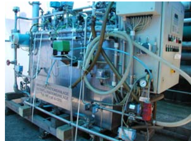
Special designed Membrane System for cleaning of Oily Water / Bilge Water
