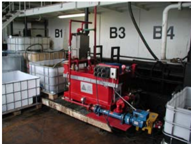
Special designed Ultrasonic Technology for cracking stabilised Oil/Water-Emulsions
