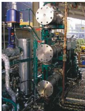
Special ESSORP -Ultrasonic-Technology for cracking stabilised Oil / Water-Emulsions
