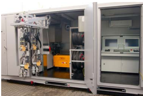
Control Room with Manway Cannon ready for operation
