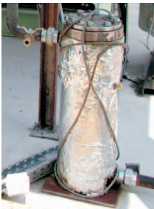
Special ESSORP -Ultrasonic-Technology for cracking the Emulsions
