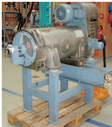
ESSORP -3-Phasen-Decanter, for separation of oil, water & solids
